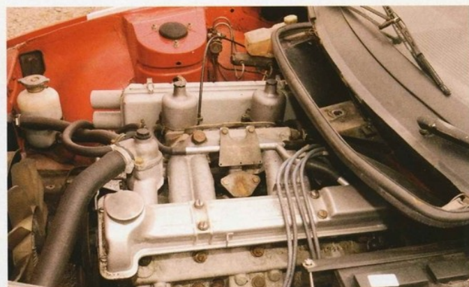
Above: Two-litre, slant four-cylinder engine has a heavy-duty alternator to cope with the demands of the extra accessories, but is otherwise standard. Car is also fitted with air-conditioning
